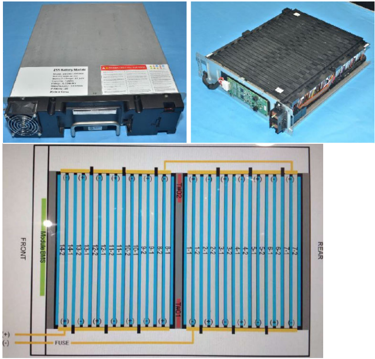
Figure 16 A description of the battery cell numbering in the LG Chem battery modules. Battery 7 is the last two cells (pair); 7-1 is next one inward, 7-2 is rearmost (image credit: APS)
