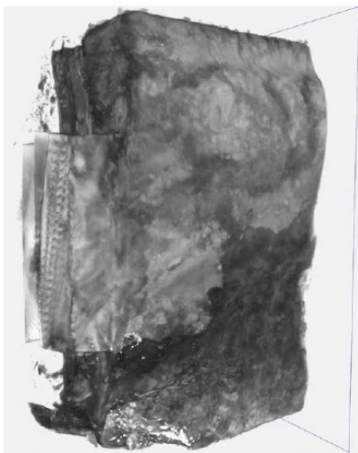
Figure 18 A 3D reconstructed image of the CT-scanned battery cell 7-2 demonstrates the absence of material in the bottom corner of the battery cell (image credit: SEL)
