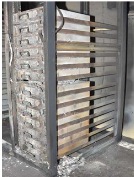
Figure 23 All of the modules in Rack 15 were damaged by thermal runaway while leaving the neighboring racks mostly undamaged (image credit: APS)
